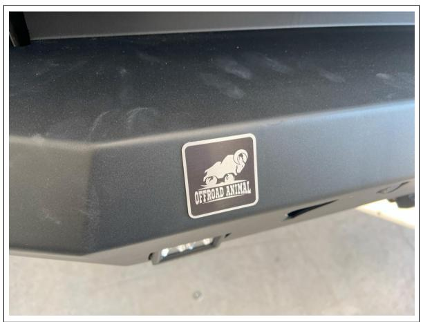
45. Attach Offroad Animal Logo plate to chamfered face, using attached adhesive backing.
