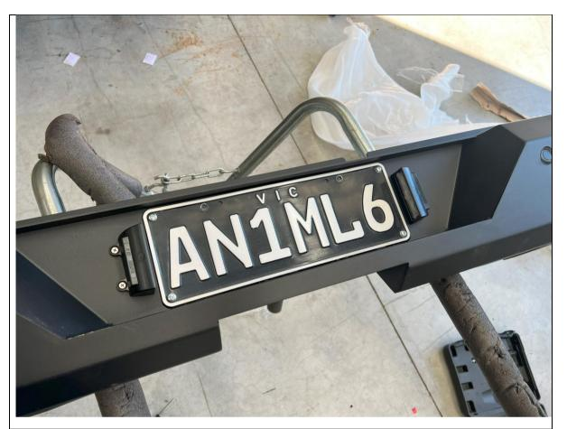
33. Re-Fit number plate to the bar, using supplied M5 Fasteners.
